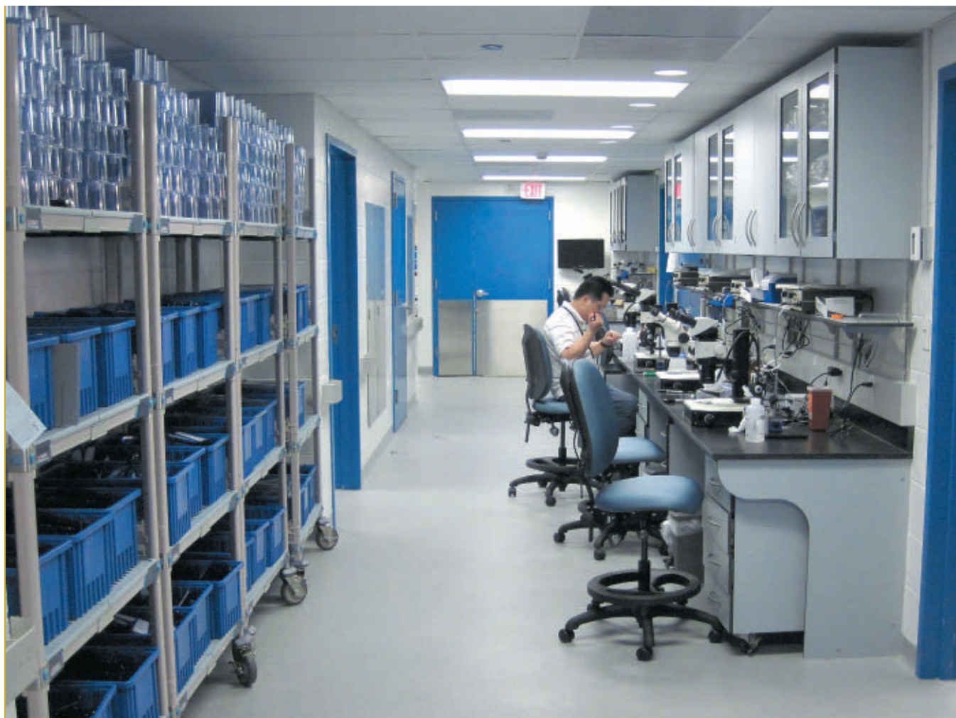
Extensive work areas for researchers lie only a few feet from the fish housing rooms. They feature fiberglass doors, phenolic casework with epoxy work surfaces and epoxy floors and walls. Image: Erik Sanders
